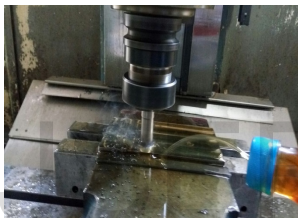
Fig.1. Machining of work piece by applying parameters – Spindle Speed 1800rpm, Feed Rate – 200mm/min and Depth of Cut – 0.5mm, Solid Carbide Tool, Cutting Fluid – Semi Synthetic oil
